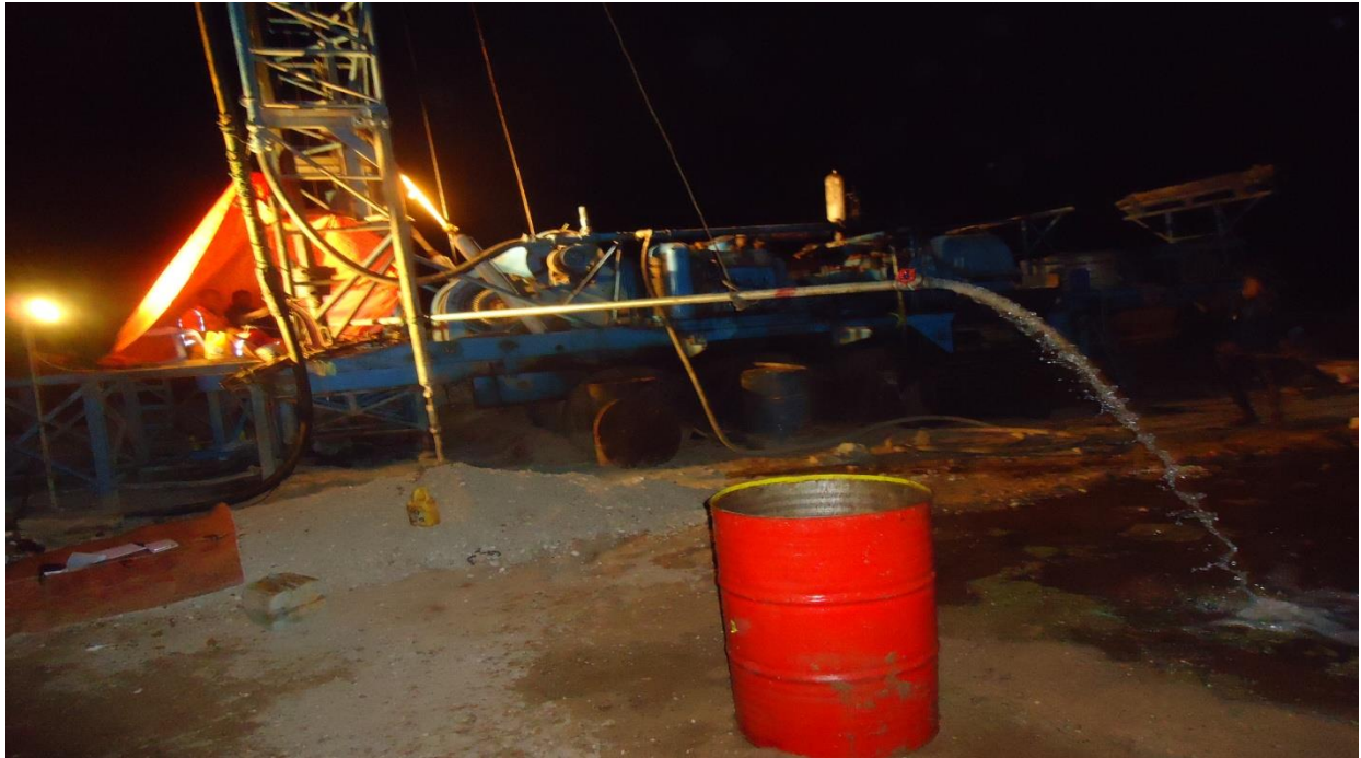
Awrculus Borehole, During pump Test process 253m deep and yield of 11m 3 funded by ICRC
